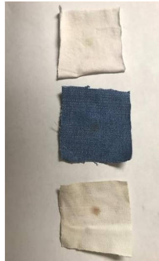
Fig. 2. Group 1 after having undergone the stain removal treatment and dried with the cotton fabric on the top, denim in the middle, and canvas on the bottom.
