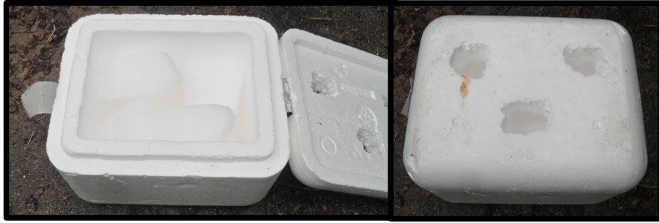
Fig. 2. From left to right, dry ice after being cut and placed into the cooler and a foam box with three 5.08 cm diameter holes in the lid to allow CO 2 gas to escape.
